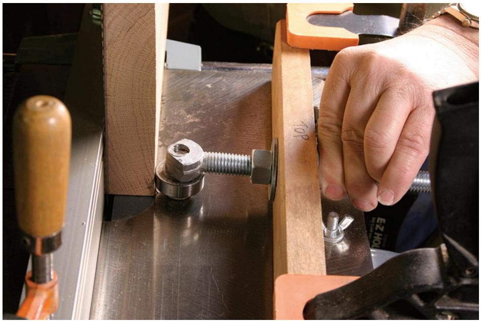
6. Loosen the jam nuts and move the threaded part of the jig up against the work you are going to be resawing – trapping it between the jig's bearing and your band saw's fence. Note that the bearing should be positioned so it's 1/4" to 1/2" in front of the teeth of the saw's blade.
