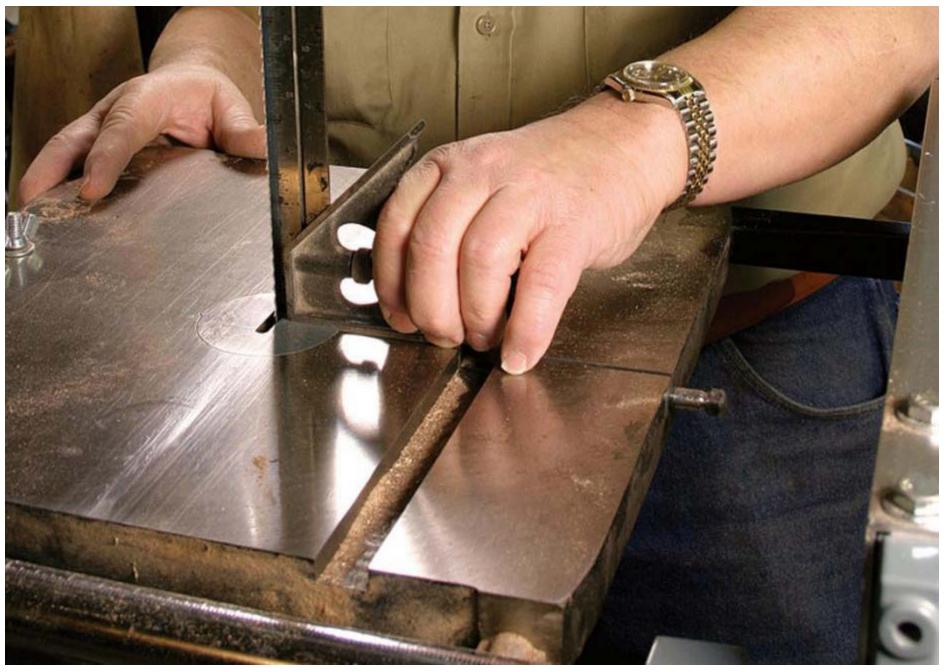
1. First tension your blade. I use a 1/2"-wide blade and tension it so the indicator of the saw reads 3/4". Ensure your band saw's table is square to the blade. Raise the blade guides up as far as they will go and check the blade with a square.
