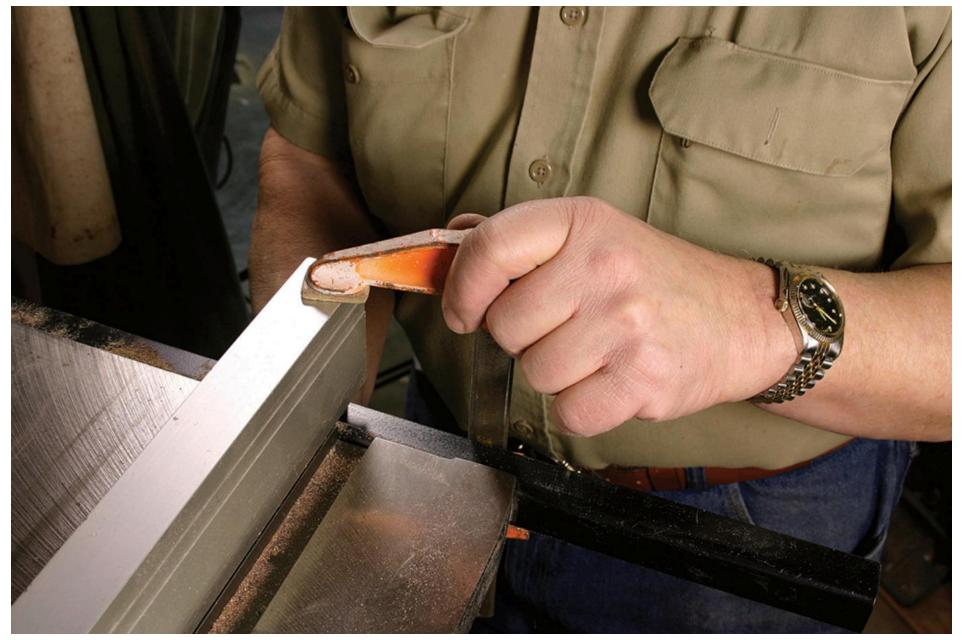
2. Set the fence parallel to the blade. The distance between the blade and the fence should be the thickness of the veneer you want to slice. I set the fence to the right of the blade so it feels more like a table saw and clamp the outfeed end of the fence to the table.
