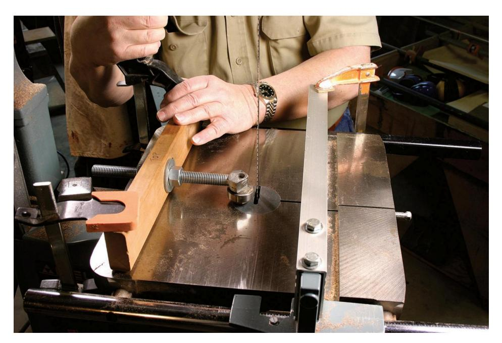
5. Here, you can see how my simple little jig works. The threaded section is a common \$9 hinge (called a bolt hook) for a farm gate that I modified. I sawed off a vertical pin on the end of the hinge, then I bored a hole at one end and bolted a 1 1/8"-dia. bearing to the hinge (any diameter bearing will work as long as it clears the hinge). The bolt head rests on the machine's table. The threaded section of the hinge is held in place by two jam nuts and washers.
