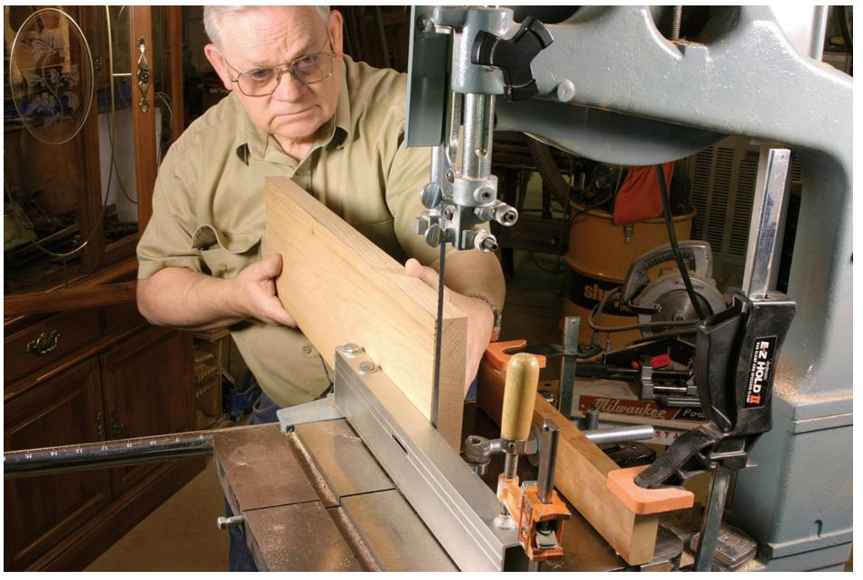
7. Turn on the saw and make a test cut. Push the work through firmly but don't stress the motor. If you've set your jig correctly, you'll slice off perfectly consistent pieces of veneer. After your first cut, reset the jig's bearing against your next piece of work and make your next cut.
